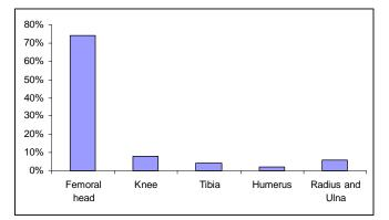
**Fig. (4b).** Failure of SS implants at various anatomical locations (Ref. Sivakumar M, Suresh Kumar Dhanadurai K, Rajeswari S, Thulasiraman V. Failures in stainless steel orthopaedic implant devices: a survey. J Mater Sci Lett 1995; 14: pp. 351-4).
