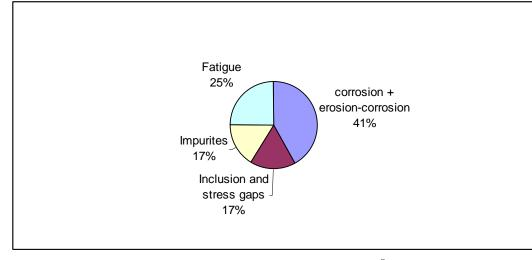
Fig. (3). Failure analysis of implants Ti6Al4V and 316L steel. Ref: Aksakal B, Yildirim ÖS, Gul H. J Fail Anal Prevent 2004; 4(3): p. 17].
