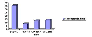
**Fig. (2).** Regeneration time of surface oxide films for various alloys. [Ref: Hanawa T. Reconstruction and regeneration of surface oxide film on metallic materials in biological environments. Corrosion Rev 2003; 21: pp. 2-3].
