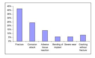
Fig. (4a). Causes for failure of SS implants.
